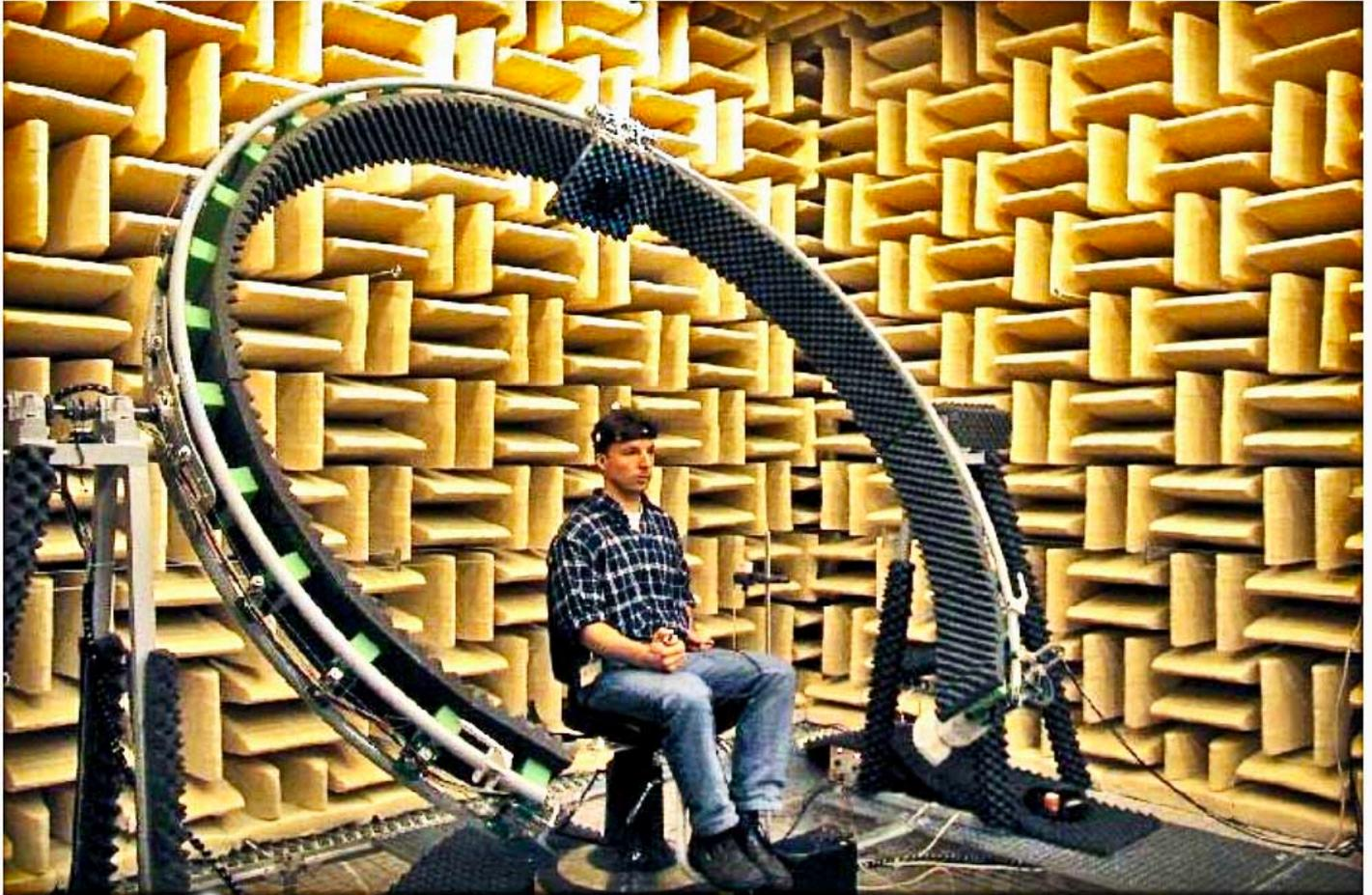
**Setup for measuring head-related transfer functions**
